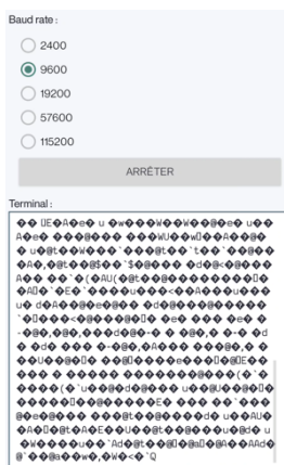
Figure 3. Baud rate incompatible
